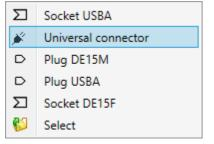
The connector will follow the cursor and must be placed on the page. The principle and possibilities of orientation of connector in the device are the same as for the individual contacts (see above). It should be borne in mind that for connectors from the library, contacts are placed on the column with contact numbers.
